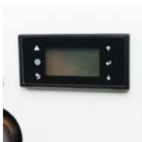
Integrated digital chiller control/display.
